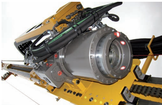
KH 9SK HDI-Ausrüstung KH 9SK jet grouting equipment
